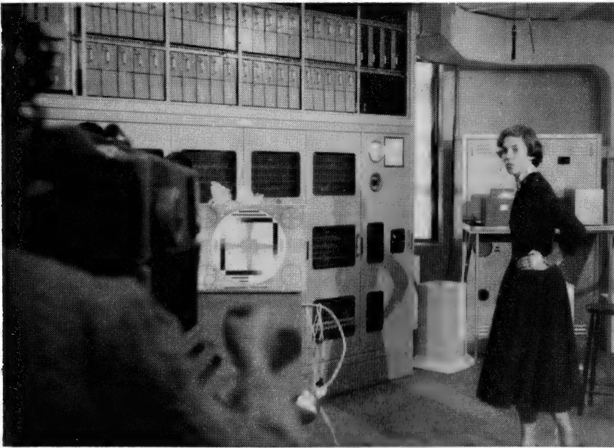
The venerable SILLIAC (Sydney University's ILLIAC I), which had the unlikely word length of 42 bits. (Note 'Auntie Marge' in the New Look — hemlines keeping up (or down) with word lengths.)
