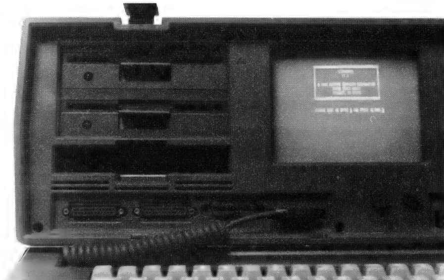
A close-up of the Executive's disk drives, screen, and peripheral connections.
