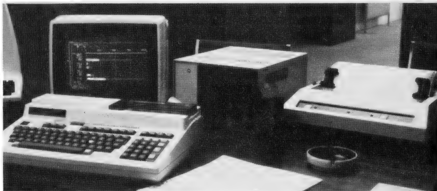
A complete Sord M23 system with keyboard, monitor, disk drives and printer.
