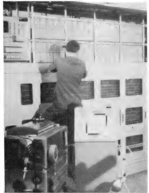
The venerable SILLIAC (Sydney University's ILLIAC I), which had the unlikely word length of 42 bits. (Note 'Auntie Marge' in the New Look — hemlines keeping up (or down) with word lengths.)
